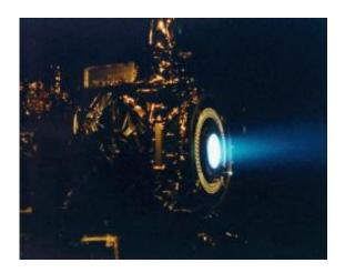
Unconventional engine: An ion engine provides Dawn with the propulsion it needs. Credit: Nasa/JPL
