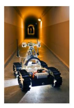
Sandia's Gemini-Scout Mine Rescue Robot is equipped to handle any number of obstacles, including rubble piles and flooded rooms, to help rescuers reach trapped miners safely and efficiently. Credit: Randy Montoya
