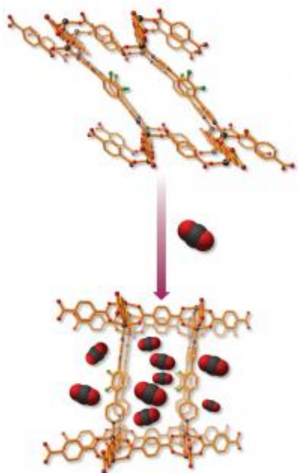
Figure 1: In the presence of carbon dioxide molecules (red and black), the molecular PCP cage expands to adsorb the gas. Credit: 2011 Ryotaro Matsuda
