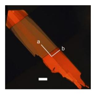
A single crystal of the new organic semiconductor material shown in polarized light. It is approximately twice as fast as the parent organic material from which it was derived. The white scale bar at the bottom center of the photo represents 10 microns (10 millionths of a meter).
