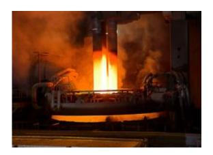
Contact-free measurement of the temperature of molten steel boosts the productivity of arc furnaces. That's why Siemens has developed a system called Simetal RCB Temp, which consists of an optical sensor that can determine the temperature of the molten metal in the steel production process (over 1,500 degrees Celsius) at shorter intervals than was previously the case. As a result, the best time to tap can be determined more exactly, thus saving time and energy and increasing work safety.
