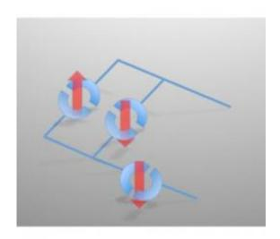
In future, X-ray beams could be used to write superconducting circuits, such as those depicted in the image. Here, solid lines indicate electrical connections while semicircles denote superconducting junctions, whose states are indicated by red arrows. Credit: UCL Press Office
