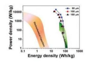
Compared with supercapacitors and batteries, SMCs (with three different electrode thicknesses shown) offer both a high power density and high energy density. Image copyright: Jang, et al. ©2011 American Chemical Society
