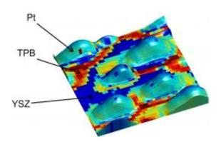
A new ORNL microscopy technique allows researchers to study key reactions in fuel cells at an unprecedented scale. The overlay shows electrochemical activity of platinum (Pt) nanoparticles on an yttria-stabilized zirconia (YSZ) surface, revealing enhanced activity along the triple-phase boundaries (TPB). Credit: ORNL
