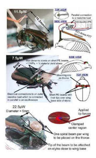
Three energy-scavenging prototypes: (Top) A piezoelectric cantilever beam attached lengthwise along the beetle's body generates 11.5  $\mu$ W. (Middle) Piezoelectric cantilever beams attached across the beetle's body each generate 7.5  $\mu$ W. (Bottom) Piezoelectric spiral beams attached on the beetle's thorax each generate 22.5  $\mu$ W. Image credit: Aktakka, et al.
