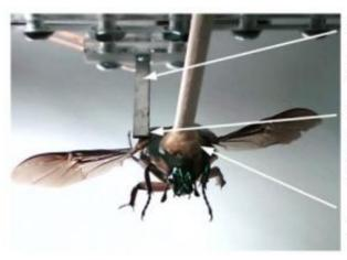
Piezoelectric Cantilever Beam Resonance freq. = 423 Hz Spring constant = 407mN/mm
