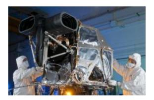
The Operational Land Imager (OLI), built by the Ball Aerospace and Technologies Corporation, will fly on the Landsat Data Continuity Mission. OLI will measure in the visible, near infrared, and short wave infrared portions of the spectrum, with an improved signal-to-noise ratio compared to past Landsat instruments. The opening facing the left of the photo will point at the Earth, and the opening on the right is for pointing towards the sun, to calibrate the instrument. Credit: Ball Aerospace
