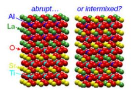
Is the interface of insulating lanthanum aluminate (LaAlO3) and strontium titanate (SrTiO3) abrupt or intermixed? This question is answered in studies using pulsed laser deposition and x-ray photoelectron spectroscopy at EMSL.
