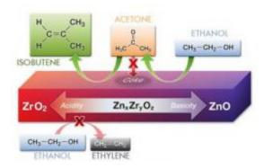
The right balance of zinc and zirconium oxides in this catalyst (purple block) converts ethanol to isobutene with low amounts of unwanted byproducts such as acetone and ethylene. Credit: PNNL
