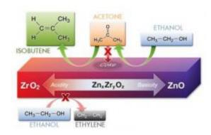
The right balance of zinc and zirconium oxides in this catalyst (purple block) converts ethanol to isobutene with low amounts of unwanted byproducts such as acetone and ethylene. Credit: PNNL
