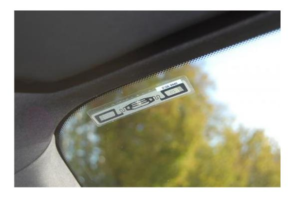
The RFID chip is affixed on the inside of the windshield. It measures just 1.5 x 10 centimeters. (© motionID technologies)
