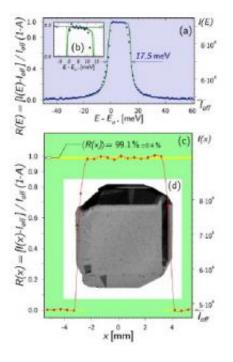
Absolute reflectivity of 13.9-keV x-rays from the (008) atomic planes of a diamond crystal in Bragg backscattering (a)-(c), and x-ray Lang transmission topogram of the diamond crystal (d). The diamond crystal, nearly defect-free in a volume of 5 x 5 x 1 mm3, reflects more than 99% of hard x-ray photons backwards in Bragg diffraction, with a remarkably small variation in magnitude across the sample.
