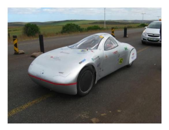
They traded off comfort, being a single-seat experimental car, for reduced weight. The designers made use of two wheel-mounted hub-motors. There was no need to accommodate an internal engine or transmission. Their design represents a lighter vehicle with an efficient battery management system which evenly divides the load among 14 individual lithium-cobalt battery packs.
