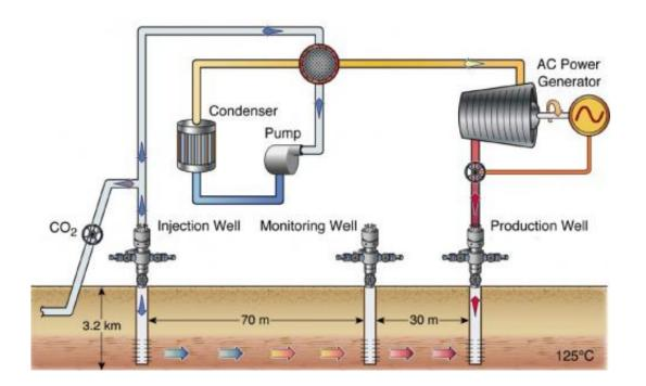
This looks like a maze, but it's actually a schematic of a way to combine CO2 storage and geothermal energy production. Starting with CO2 on the left, follow the arrows to learn how the proposed pilot test will work.
