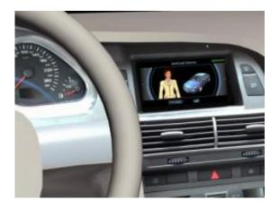
Displayed on the monitor of the Audi Mulitmedia Interface that comes standard in all new Audi models, an avatar supports the driver with explicit information on the vehicle in a natural-language dialog -- supported by images and videos. The system can be triggered by spoken questions or by touching controls, making cumbersome paging through owner's manuals a thing of the past. Credit: Institute of Business Informatics, Technische Universitaet Muenchen
