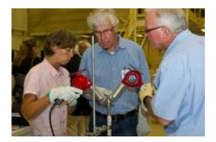
From left to right: Petra Neuhause and Harold Lenski, both with Astrium, Germany accompanied by Jeff Clancy of Teledyne Brown Engineering, use a heat gun to open the first U.S. sample cartridge processed in the solidification quench furnace in the Materials Science Research Rack aboard the International Space Station. The sample was returned to Earth on the space shuttle mission STS 133. Credit: NASA/MSFC/Emmett Given
