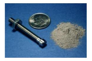
This finished 1.8 gram titanium bolt is made from 1.8 grams of gas atomized titanium powder. Iowa Powder Atomization Technologies produces the titanium powder, using technology licensed from the US Dept. of Energy's Ames Laboratory. Credit: U.S. Dept. of Energy's Ames Laboratory.
