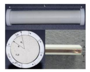
Photographs of: (top) the assembled cloak on the test cylinder with end caps; (bottom left) a cross-section view of the assembly with end cap removed; (bottom right) a shell segment edge with copper tape used to form the metallic strip for the metamaterial cloak. Image from arXiv:1107.3740v1
