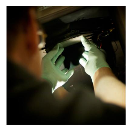
Barr places a sheet of paper with a mask on it into the vapor-printing chamber. *Photo: Patrick Gillooly*
