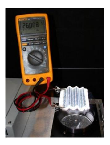
A paper solar cell that has been repeatedly folded is illuminated from below and connected to a voltmeter to demonstrate its output (26 V). Image courtesy of the Gleason Lab
