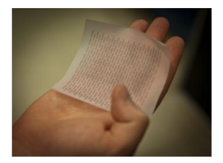
Barr holds a sheet of paper that has had one of the layers of the solar cell printed on its surface. Photo: Patrick Gillooly
