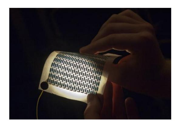
Graduate student Miles Barr hold a flexible and foldable array of solar cells that have been printed on a sheet of paper. *Photo: Patrick Gillooly*
