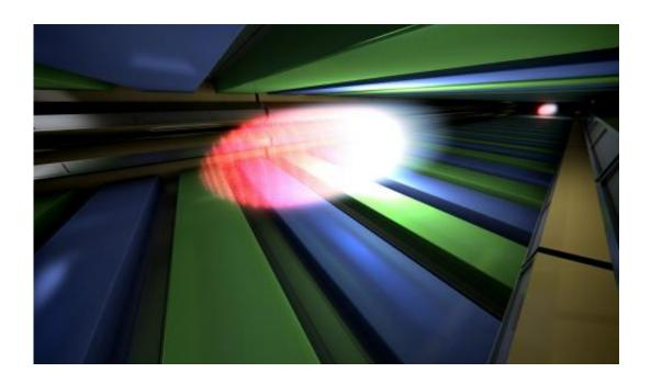
Generation of X-ray laser flashes in an undulator. To generate the extremely short and intense X-ray laser flashes, bunches of high-energy electrons are directed through special arrangements of magnets (undulators). Credit: European XFEL
