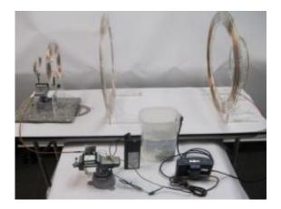
The experimental setup has a large transmission coil, at the right, connected to the building's electricity. At the left is the receiving coil, and near it is a smaller coil connected to a commercial heart pump sitting in a jar of fluid. Credit: University of Washington
