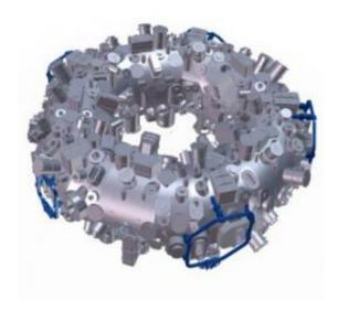
The outer vessel of Wendelstein 7-X equipped with a variety of ports. Blue: five auxiliary coils, which are provided by Princeton Plasma Physics Laboratory. They are to help precise setting of the magnetic fields at the plasma edge. Credit: (Graphic: IPP)
