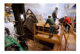
After pouring more than 7,000 pounds of molten aluminum on June 16, 2011, workers at Portage Casting and Mold Inc. in Portage, Wis., open a five-section-mold that formed one of two nine-meter-diameter hemispheres needed for the main vacuum vessel of the Plasma Dynamo Facility being installed at Sterling Hallon campus. Photo: Jeff Miller
