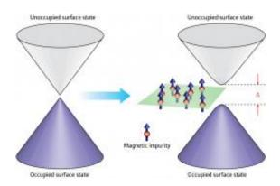
The introduction of magnetic impurities into a topological insulator causes a gap to open in the characteristic double-cone energy structure of the material (the x-axis shows electron momentum, the y-axis shows the energy). Credit: 2010 AAAS
