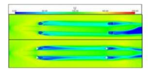
In simulations conducted at the Ohio Supercomputer Center, Ohio State University engineering students compared the airflow under the Buckeye Bullet traveling at 300 mph without wind deflectors installed in front of the wheel wells (above) with the airflow under the vehicle with wind deflectors installed (below). Credit: Center for Automotive Research at the Ohio State University
