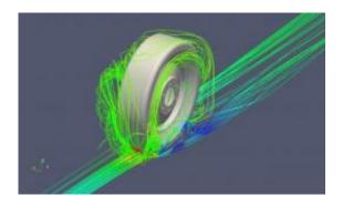
In a simulation run by Ohio State University student engineers at the Ohio Supercomputer Center, an isolated view of a wheel on the Buckeye Bullet illustrates airflow within the wheel well with the vehicle traveling at 300 mph. Credit: Center for Automotive Research at the Ohio State University
