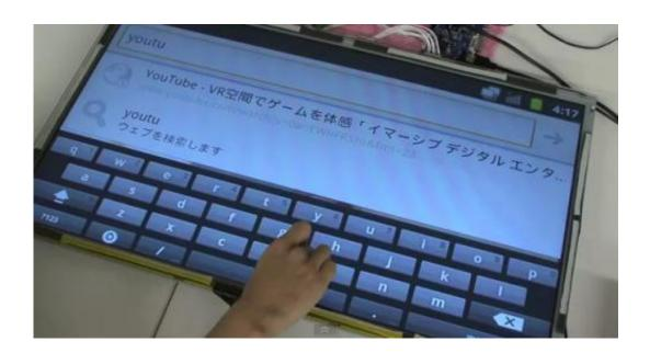
(PhysOrg.com) -- Researchers at SKR have developed a prototype of a multi-touch 32" display screen that runs on the Android operating system. The screen, which runs off of a standard Android terminal, is connected to the touch sensors and an HDMI screen via a USB port. The end result of the screen is that the android interface works like smaller devices, but it can also display large format Full HD video.
