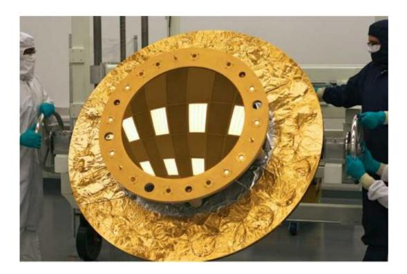
The secondary mirror (shown here) was polished at the L3 Integrated Optical Systems - Tinsley in Richmond, Calif. to accuracies of less than one millionth of an inch. That accuracy is important for forming the sharpest images when the mirrors cool to -400°F (-240°C) in the cold of space. The Webb's secondary mirror was recently completed, following polishing and gold-coating. Credit:NASA/Ball Aerospace/Tinsley
