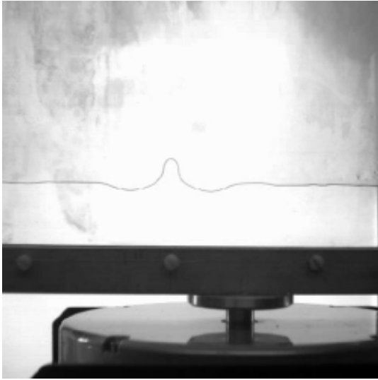
The even standing solitary wave. Video copyright: Jean Rajchenbach, et al. ©2011 American Physical Society
