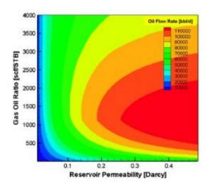
Among their findings, the Berkeley Lab team found that reservoir permeability had a strong influence on oil flow rate. This graphic tracks oil flow rate, in barrels per day, as a function of reservoir permeability and gas-oil ratio in a model in which the pressure at the blowout preventer is 4,400 pounds per square inch.
