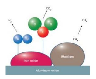
Schematic illustration of a rhodium-iron oxide catalyst on solid aluminium oxide for converting bioethanol into hydrogen gas at low temperature. Credit: The Agency for Science, Technology and Research
