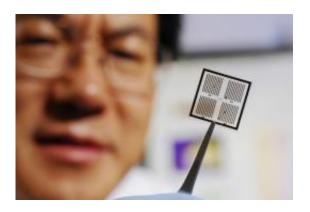
Regents professor Zhong Lin Wang holds an array of piezoelectrically modulated resistive memory (PRM) cells on which metal electrodes have been patterned using lithography. Credit: Gary Meek
