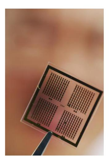
Image shows an array of piezoelectrically modulated resistive memory (PRM) cells on which metal electrodes have been patterned using lithography. Credit: Gary Meek
