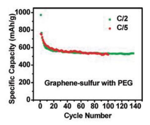
The cycling performance of the PEG-coated graphene-sulfur composite shows that it can maintain a specific capacity of close to 600 mAh/g for more than 100 cycles. Image copyright: Hailang Wang, et al. ©2011 American Chemical Society
