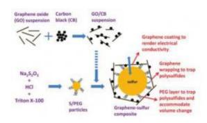
Synthesis steps for a graphene-sulfur composite, which can be used as a cathode material for rechargeable lithium-sulfur batteries with a high energy density. Image copyright: Hailang Wang, et al. ©2011 American Chemical Society
