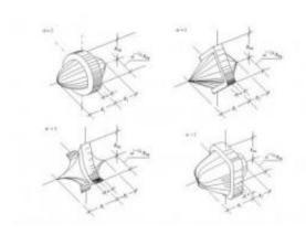
When "designer" particles like these are placed next to one another, the way mechanical energy travels through them is profoundly affected, according to new University at Buffalo research. Crafting such designer particles would enable scientists and engineers to control how energy travels through a granular system. Credit: Surajit Sen, University at Buffalo
