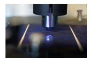
Inside the FlashQE, developed at NREL, light from light-emitting diodes is focused onto a solar cell. Credit: Dennis Schroeder
