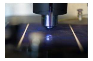
Inside the FlashQE, developed at NREL, light from light-emitting diodes is focused onto a solar cell. Credit: Dennis Schroeder
