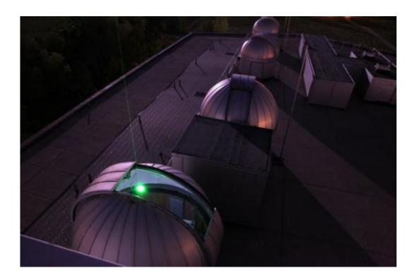
Lidar instruments - pointing up from the ground or down from satellites - use reflected light to measure the amounts of particles and their locations, which can influence climate. (Credit: CIRES/NOAA)
