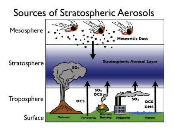
Sources of aerosols reach the stratosphere from above and below, as shown in the graph. Sulfur dioxide (SO2), carbonyl sulfide (OCS), and dimethyl sulfide(DMS) are the dominant surface emissions which contribute to aerosol formation. (Credit: NOAA)
