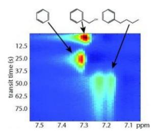
This 2-D plot shows separation of benzyl alcohol, benzene and butylbenzene using remote NMR/MRI with a monolithic chromatography column. Horizontal axis corresponds to the NMR chemical shift, vertical axis represents the transit time of compounds undergoing chromatographic separation. Credit: Alex Pines group
