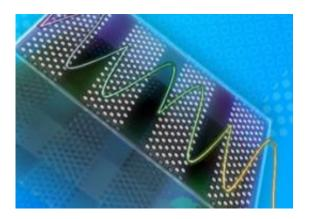
In this illustration, light hits Kocaman's and Wong's specially engineered material without leaving a trace. The actual material is no thicker than one hundredth of the diameter of a strand of hair.
