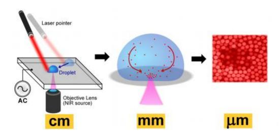
This graphic illustrates a new technology that combines a laser and electric fields to manipulate fluids and tiny particles such as bacteria, viruses and DNA for a range of potential applications from drug manufacturing to food safety. The technologies could bring innovative sensors and analytical devices for "lab-on-a-chip" applications. Credit: Stuart J. Williams, University of Louisville
