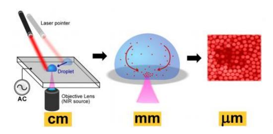
This graphic illustrates a new technology that combines a laser and electric fields to manipulate fluids and tiny particles such as bacteria, viruses and DNA for a range of potential applications from drug manufacturing to food safety. The technologies could bring innovative sensors and analytical devices for "lab-on-achip" applications. Credit: Stuart J. Williams, University of Louisville
