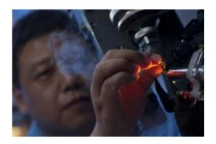
Rice University postdoctoral researcher Jinhui Dong mounts a protein crystal to an X-ray machine to collect diffraction data. Credit: Jeff Fitlow/Rice University
