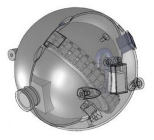
A spherical robot equipped with a camera may navigate underground pipes of a nuclear reactor by propelling itself with an internal network of valves and pumps. Image: Harry Asada/d'Arbeloff Laboratory
