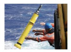
Deploying an Argo ocean profiler. Credit: CSIRO
