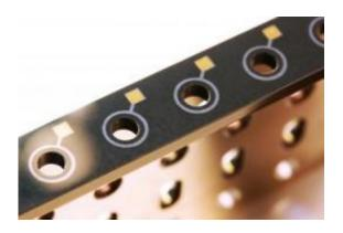
This tailpiece is coated with a thin-film sensor system. It converts the tension on the string into digital control signals. Credit: © Fraunhofer IST
