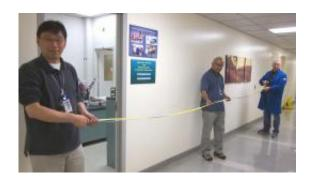
ORNL researchers (from left) Zhili Feng, Stan David and Alan Frederic display a length of wire more than 15 feet long fabricated with the friction-stir extrusion method. They eventually ran out of the magnesium-aluminum alloy feed stock. Friction-stir extrusion is an energy-efficient method for making wire from high-temperature, recyclable materials.
