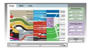
The Foreseer tool is based on Sankey diagrams, where the width of each line is proportional to the quantity of resource. Credit: The Forseer Project
