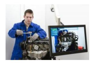
The system uses the 2-D barcodes attached to various parts of the malfunctioning machine to determine the camera's position and direction of view and then sends this data to the experts. Credit: © Fraunhofer FKIE
