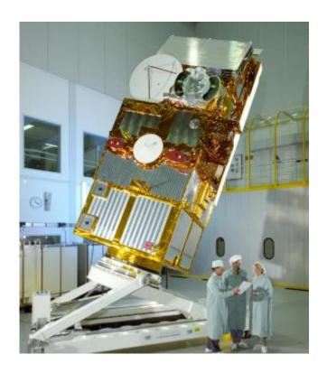
ERS-2 satellite prior to launch. ERS-2 was launched in 1995, following its sister, the first European Remote Sensing satellite ERS-1, which was launched in 1991. The two satellites were designed as identical twins with one important difference - ERS-2 included an extra instrument to monitor ozone levels in the atmosphere. Credits: ESA
