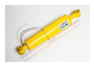
The shock absorber harvests energy from vibrations experienced by a vehicle's suspension system into electricity that can charge the battery and power vehicle electronics. Image credit: Lei Zuo
