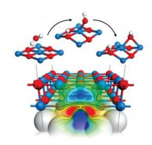
Figure 1: Defects inside an ultrathin magnesium oxide film (red and blue spheres, bottom) accumulate electronic charges (red and blue contour map) and enhance the catalytic dissociation of water molecules (top). Credit: 2011 Yousoo Kim
